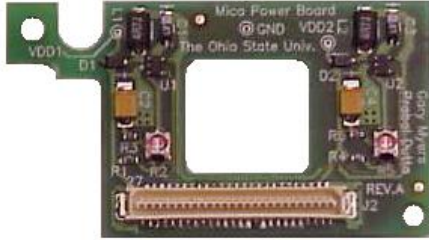
Figure 3: The Mica Power Board has two fully independent switching regulators that are potentiometer adjustable and can deliver 3V - 40V at 200mA each. The odd shape of this board is reflects the need for physically compatibility with the Mica Sensor Board.
