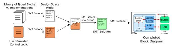
Figure 3: Design Generation at a High Level. EDG tools use existing constraint solvers to perform synthesis. The tools convert knowledge about the design space and control logic specification into constraint satisfaction problems whose solutions are block diagrams describing valid device designs. These block diagrams completely specify the design of an embedded device and can be easily converted to more useful formats.
