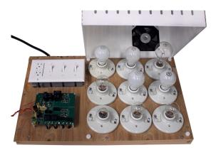
Figure 7: Calibration testbed. A control board manages nine circuits of light bulbs and power resistors with varying wattages. The values are chosen to allow for 1 W steps in load power. Light switches provide a hard shutoff, but during experimentation, wattages are selected via relays controlled by an Epic Core on the control board shown in the bottom left. The load is independently metered by a PLM-1LP for ground truth.
