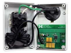
Figure 19: Monjolo sensor in plug-load form. The case is open so that the female socket is visible on the left and the male plug is visible on the right. The energy-harvesting power supply is visible in the lower right PCB. The Epic Core is attached to the opposite side of the same PCB.
