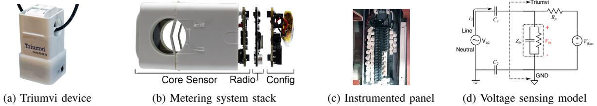
Fig. 2: Sensor implementation, composition, deployment, and equivalent circuit for non-contact AC voltage sensing.
