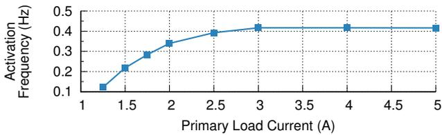
Fig. 10: Activation rate as a function of primary load with power factor of 1.0. Below 1.25 A, the meter is unable to harvest enough power to measure, but at 3 A it can sample at nearly 0.5 Hz.
