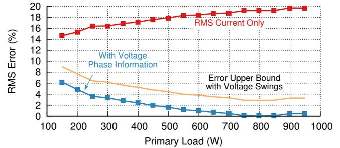
Fig. 14: Error with and without voltage phase information. For a range of loads with power factor of 0.85, the RMS error of Triumvi’s power measurement using only RMS current and using sampled current plus voltage phase information is shown. Without any voltage information the error averages 18.5% RMS, and with phase information the average error is 2.5% RMS.
