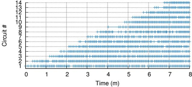
Fig. 16: Installation time for 14 circuits. As Triumvi devices are configured with the panel ID and circuit number, and clipped around the correct circuit, they begin transmitting measurements. Each mark represents a received packet. Based on the start time of the circuit #14, installing 13 meters took about seven minutes for a familiar, but inexperienced user. Overall, we expect deployments to take a half hour or less.
