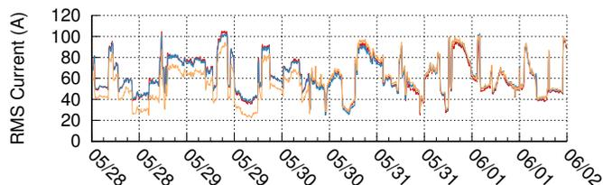
Fig. 18: Triumvi measurements of a large water pump. The 1000 A Triumvi variant with 3-phase synchronized measurements meters a municipal water pump for five days. The load phases were unbalanced and subsequently fixed, and Triumvi correctly detected this as confirmed by the water utility.
