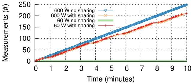
Fig. 11: Example of charge sharing between meters on a 600 W load and a 60 W load. The meter on the higher load drops from a sample rate of 0.42 Hz to 0.35 Hz, but by sharing its charge the meter on the 60 W load goes from being unable to charge to a sample rate of 0.35 Hz. Charge sharing is an effective way of mitigating the minimum load requirement of energy-harvesting without requiring battery or mains power.
