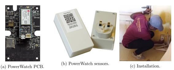
Figure 4.1: **PowerWatch as deployed.** (a) PowerWatch PCB with cellular radio, SD card, and sensing circuits. (b) Assembled PowerWatch sensors with QR code scanned at installation to associate the sensor with a participant. (c) A field officer installing a PowerWatch sensor at a household outlet.
