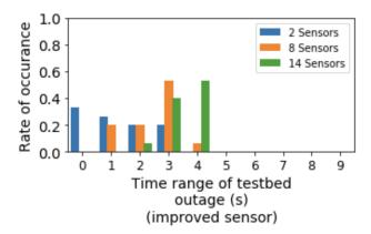
Figure 4.8: **Time range of testbed outages with improved firmware.** Improved firmware decreased the variance to closer to what would be expected, although leaving room for improvement in firmware optimization.
