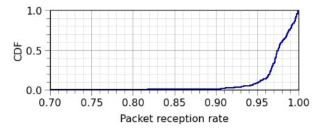
Figure 4.10: **Packet Reception Rate (PRR).** PRR was calculated by comparing each sensor's expected reporting interval and sequence numbers with data received. Jumps in sequence number, or periods sensors did not report when expected, indicated a transmission failure due to lack of cellular connection or bugs in the firmware. Sensors were not included after permanent failure, and PRR was increased by local queuing.
