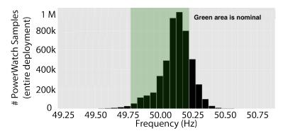
Figure 5.11: **Frequency in sample is unstable.** We see that while a majority of our samples are within the acceptable range around the nominal 50 HZ, there are still a significant number of readings that represent deviations beyond the acceptable range of 49.8 to 50.2 HZ.
