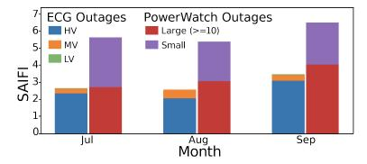
Figure 5.5: Comparison of PowerWatch S-SAIFI to the utility-reported SAIFI in quarter 3 of 2018. Our large outage clusters closely compared to the combined medium-and high-voltage SAIFI reported by ECG, while low-voltage outages (small outage clusters) sensed by PowerWatch greatly exceeded low-voltage SAIFI reported by ECG. This provides evidence of the extent of under-sampling by the utility at the low-voltage level of the grid.
