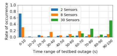
Figure 4.7: **Time range of testbed outages.** A testbed of sensors and programmable outlets generated two hundred outages of various sizes in a controlled setting. We observed the precision of outage timestamping, noting that for any given outage sensors may report that the same outage occurred up to 100 s apart. This allowed us to parameterize clustering algorithms used to detect outages in the field. Newer firmware reduces temporal variance to less than 10 s.
