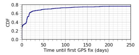
Figure 4.11: **Time to acquire first successful GPS fix.** Note CDF axis stops at 0.8. From 462 sensor deployments, over 17% achieved a fix within the first hour after their deployment began, and over 29% within the first day. Over 65% achieved a fix within 30 days. The remaining 11% that achieved a fix were spread over 300 additional days. In 23.2% of the deployments the sensors never achieved a GPS fix.
