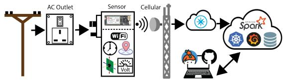
Figure 4.2: **PowerWatch System Architecture.** PowerWatch measures the grid by plugging in at outlets in homes or businesses, transmitting data about power quality over the cellular network, and clustering the data based on temporal and spatial characteristics of power outages.
