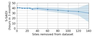
Figure 5.6: Calculated S-SAIDI  $\pm$  one standard deviation as sites are removed from the dataset between June and August 2019. To evaluate whether PowerWatch covered a sufficient sample of the grid to compute a representative S-SAIDI, we removed sites from the dataset in 30 rounds and observed the effect on S-SAIDI. We saw that as sites were removed, standard deviation of S-SAIDI remained relatively low and the mean value of S-SAIDI dropped slightly.
