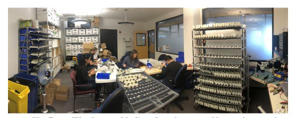
Figure 6.2: **The PowerWatch assembly line.** Over the course of four weeks, 10 undergraduates worked 110 person-hours to assemble 295 PowerWatch sensors. They were responsible for assembling the plug; screwing together the enclosure; attaching the circuit board; connecting the battery, antenna, SIM card and SD card; and provisioning the device with base firmware. They worked from team-created assembly manuals and training materials.
