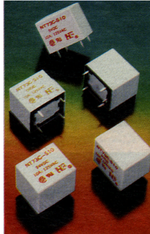
FIGURE 1. Some standard “1-Form-A” commercially available relays. Each relay is contained in a 19.6 x 16.5 x 16.5 mm non-hermetic plastic box. Minimum cost is about US$1 (in Q4 1998).
