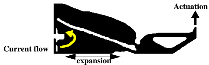
FIGURE 66. Power optimized single layer thermal bimorph actuator from [41], only the section that needs to expand carries current, reducing power usage, and the leverage system is more efficient for conversion to the desired direction.
