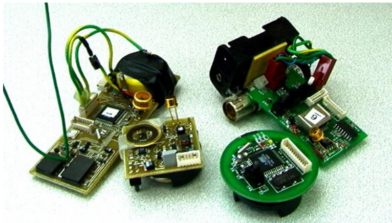
Fig. 13. COTS Motes. From left to right: RF Mote, CCR Mote, weC Mote, Laser Mote.
