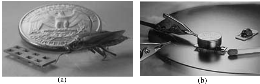
Fig. 1-5. The first walking microrobot made from polyimide thermal actuators (From Ebefors [24]).
