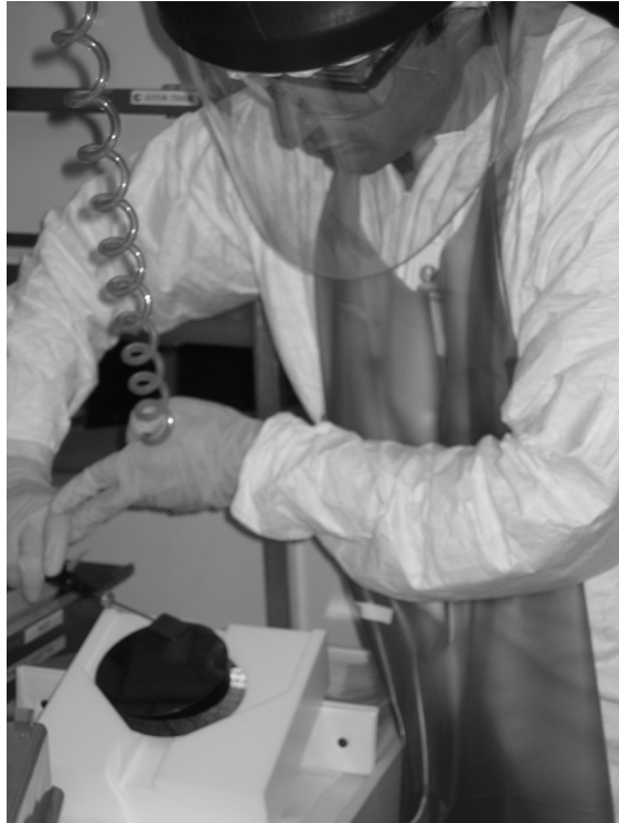
Figure 3. Making SOI wafers: Author shown bonding wafers using teflon bonding chuck.
