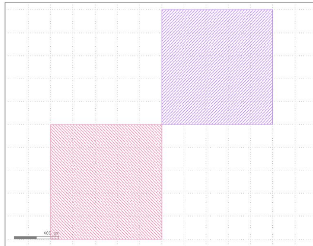
Figure 4.1: The layout file, ‘basic.gds’, that is output by the MATLAB script shown in Listing 4.1.
