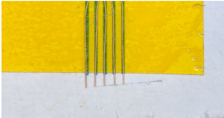
Figure 3.17: An array of lines printed onto a piece of paper used to accurately space out 60\ \mu\text{m} copper wires onto a piece of Kapton tape.
