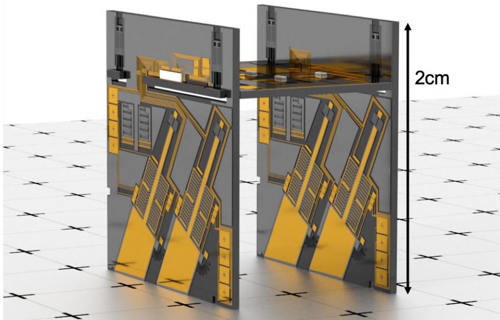
Figure 4.1: A 3D model of the walking silicon microrobot designed in this chapter. All the 3D renderings in this chapter were made using Blender.
