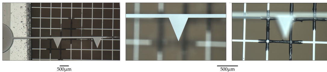
Figure 3.21: A typical failure mode of an electrode set. Permanent damage is sometimes observed following sparkover from a wire tip to the collector grid. This may be due to the relatively high current density following dielectric breakdown causing rapid Joule heating in the grid wires, or due to physical ablation during the high current breakdown. After a destructive event such as this, both electrodes were replaced despite there being no visible damage to the emitter wire.
