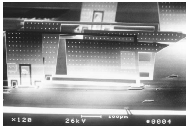
Figure 3.5: A pair of moment compensated gripper-plates. The area of the plates is 0.051 \text{mm}^2 with 500 \times 9 \times 1.5 \mu\text{m}^3 beams and an 100 \mu\text{m} gap at the base.
