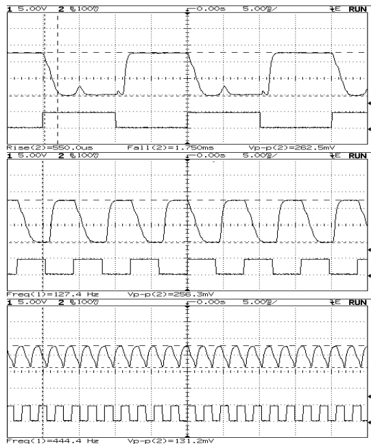
Figure 3.40: Raw output of photo detector for different CCR modulation frequencies. Direction of incident light is near (-1,-1,-1) . The square wave represents the input signal which modulates the CCR, where a low input pulls down the movable mirror. Actuation voltage is 15V.
