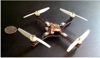
Figure 2.15: The mini quadrotor developed by Daedalus Flight Systems and UMD uses the GINA hardware, but modifies the firmware to include an onboard attitude stability loop to control its four brushless DC motors.
