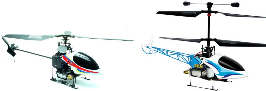
Figure 3.8: The Walkera helicopters selected as the platforms for this project are small, cheap, and commercially available 4 channel electric helicopters.
