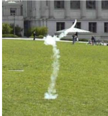
Figure 3.1: In the absence of aerodynamic forces, a bare solid rocket engine spins out of control. A stabilizing controller is therefore necessary on a minirocket LV.
