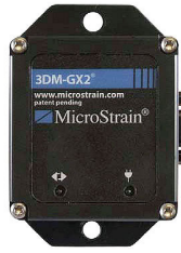
Figure 2.5: The Microstrain 3DM-GX2, a commonly used commercial IMU, can be used to calibrate and validate the performance of the GINA board
