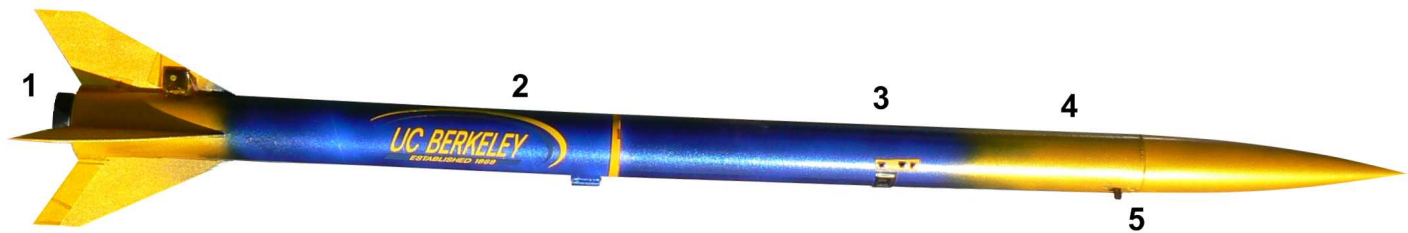
Figure 3.7: An updated rocket contained a full GINA mote for 6 axis sensing, along with 3 axis attitude control with 4 channel flywheel and gimbaled nozzle actuation.
