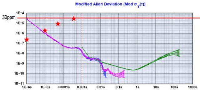
Fig. 2. Modified Allan Deviation for a temperature-compensated crystal oscillator. Line at 30ppm denotes lower limit of most specifications from Table I. Stars indicate four ways of interpreting BLE carrier drift described in Section I-A. The leftmost traces in blue and purple, terminating near 10ms and 100ms respectively, are from frequency measurements every 1 \mu s. Green rightmost trace terminating near 100s is from measurements every 1ms.
