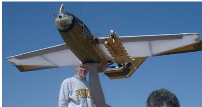
Fig. 1. Autonomous UAV with 8 wireless mesh sensors in exterior “bomb bay”. Sensors were dropped at specific GPS locations, where they formed a mesh network, shared data about vehicle magnetic events, and relayed summary track information to the UAV each time it returned and joined the network. The UAV then relayed that information to the ground station on its next overflight [1].
