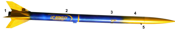
Fig. 3 Final rocket: 1) gimbaled nozzle, 2) parachute bay, 3) camera, 4) IMU, motor and payload section, 5) antenna.
