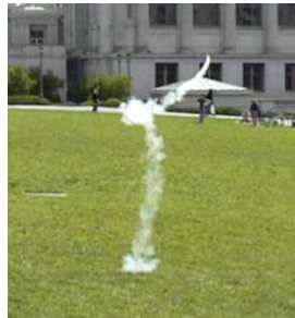
Fig. 1 In the absence of aerodynamic forces, a bare solid rocket engine spins out of control. A stabilizing controller is therefore necessary on a minirocket LV.
