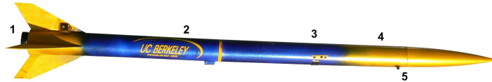
Fig. 3 Final rocket: 1) gimballed nozzle, 2) parachute bay, 3) camera, 4) IMU, motor and payload section, 5) antenna.
