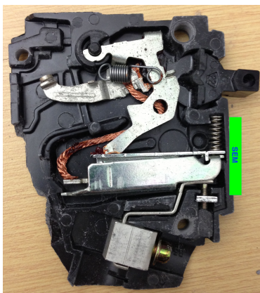
Fig. 5. Bimetallic strip circuit breaker innards with SEM annotated.
