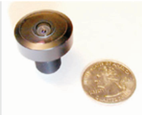
Figure 7. The OmniTech fisheye lens with 190° field of view [12].
