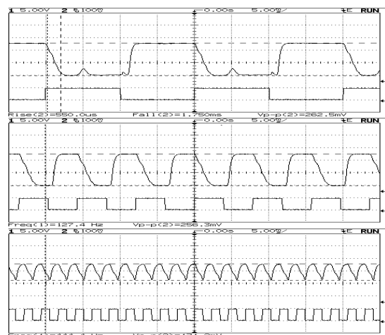
Fig. 11. Raw output of photo detector for different CCR modulation frequencies. Direction of incident light is near (-1,-1,-1). The square wave represents the input signal which modulates the CCR, where a low input pulls down the movable mirror. Actuation voltage is 15V.
