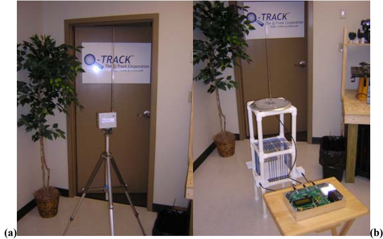
Figure 2 (a) Q-Track's prototype beacon transmitter with whip antenna. (b) Q-Track prototype locator receiver with three element array [both figures courtesy Q-Track; © 2004].
