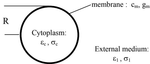
Figure 3: Protoplast model parameters
