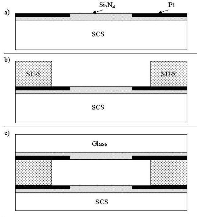
Figure 1: Micro fabrication cross-sections.
