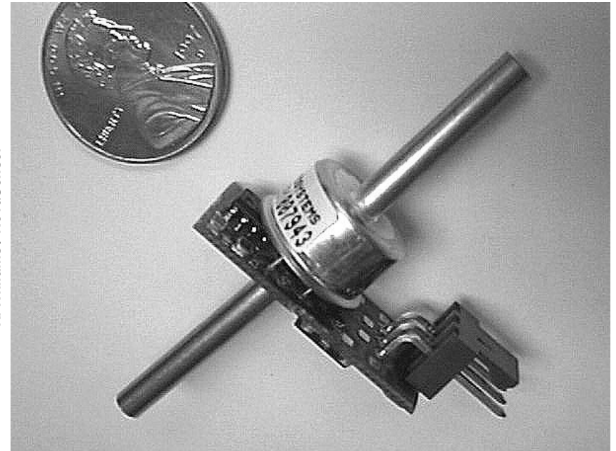
Redwood Microsystems NC-1500 Fluistor™ valve
