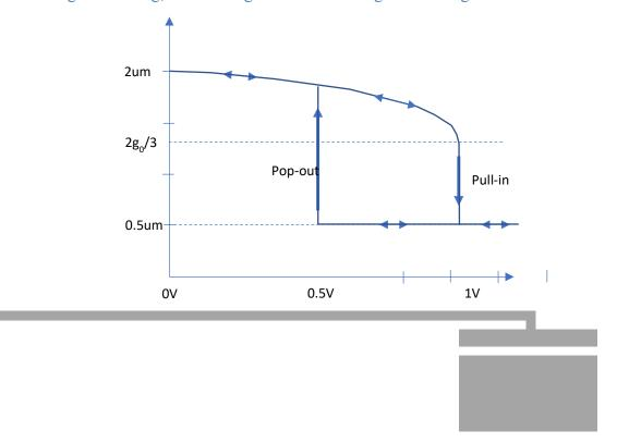
9. [4 pts total] If you were to apply a sinusoidal voltage to this structure, could you get it to pull in at a lower voltage? Why/how? What frequency would you use if you were applying a pure sine wave with no DC bias?
