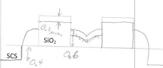
13. [6] In the following figures, a 1 micron thick SiO2 layer has been patterned to expose bare [100] silicon. Both apertures are 10um square, one is oriented in the 110 direction (parallel to the wafer flat), one is oriented in the 100 direction (45 degrees from the wafer flat). Draw the cross section after a 3 um etch in KOH.
