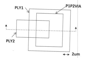
Draw a cross-section of the resulting device assuming infinite selectivity in all etches, 20% overetch in all etches except PLY2, which has 200%.
