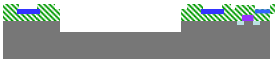
(c) A standard CMOS wafer is fabricated by an independent foundry, and cavities (mask 6) can be etched into the CMOS wafer, if needed for larger clearance under moving MEMS structures.
