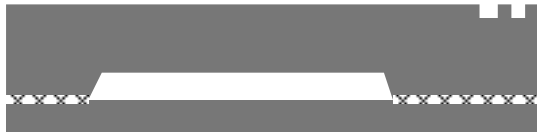
(a) The engineered silicon on insulator (ESOI) wafer is formed starting with a standard silicon handle wafer etched with simple targets for backside alignment (mask 1); followed by oxidation and cavity etch (mask 2). A second wafer is fusion bonded to the handle wafer and subsequently thinned to define the device layer thickness.
