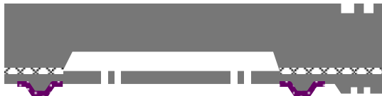
(b) The MEMS wafer is completed by etching the device layer to form standoffs (mask 3) that define the seal ring, the electrical contacts to CMOS, and the vertical gap between the CMOS and MEMS; depositing and patterning a germanium layer (mask 4) over standoffs; and patterning (mask 5) and deep reactive ion etching the device layer to form the mechanical structure.
