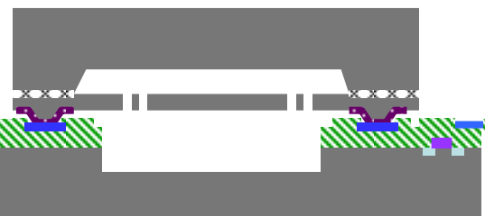
(d) The MEMS wafer is bonded to the CMOS wafer using AlGe eutectic bonding between the Al on the CMOS and the Ge on the MEMS wafer. After bonding, a portion of the MEMS wafer is removed by conventional dicing saw cuts to expose the CMOS wire bond pads.
