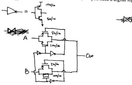
b. [2] estimate the MUX "on" resistance for an input near 0V (I want an answer in Ohms, not a formula)
