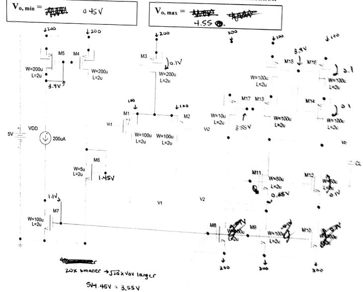
For the following problems related to the project, you will be working in a CMOS process with  $\mu_n C_{ox} = 200 \text{uA/V}^2$ ,  $\mu_p C_{ox} = 100 \text{uA/V}^2$ ,  $V_{tn} = -V_{tp} = 0.5 \text{V}$  and  $\lambda = 1/(10 \text{V}) (1 \text{um/L})$  with  $W_{min} = L_{min} = 1 \text{um}$ . Note that this is NOT the same process as you used for your project this semester.
