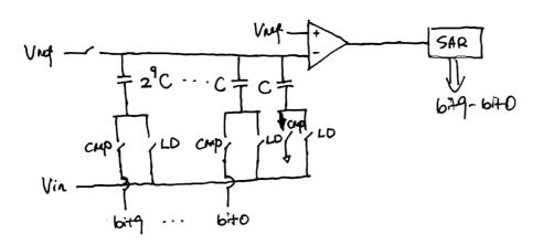
b. [2] if the unit capacitance is 2 fF, what is the total input capacitance of the ADC?
