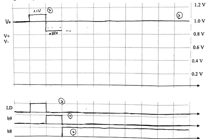
2-input MUX. Inputs will be between 0 and 1V (not 0 and  $V_{DDA}$ )
