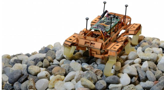
Fig. 1: Robotic platform, outfitted with motion capture tracking dots, positioned on top of the gravel used for experimentation.
