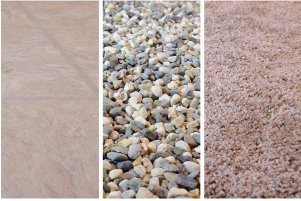
Fig. 2: Experimental test bed with interchangeable surfaces: (left) laminate tile, (middle) gravel, and (right) medium-pile carpet.
