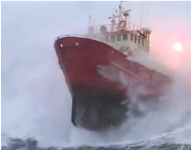
Fig. 1. A ship in high sea. The wave forces can result in very high accelerations in the ship motion. (©2010 IEEE)
