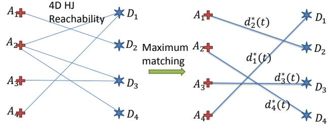
Fig. 2: The 4D HJ reachability and maximum matching approximation to the multiplayer reach-avoid game. A maximum matching of size  $m$  indicates that at most  $N - m$  attackers will be able to reach the target.
