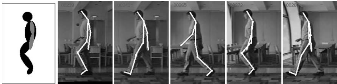
Figure 2. Example configurations of the estimated kinematic structure. First image shows the support maps of the initial configuration. In subsequent images the white lines show blob axes. The joint is the position on the intersection of two axes.
