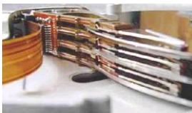
Read/Write Head Side View
