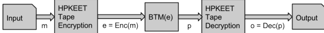
Figure 2: Overview of how the system works: The BTM (BlindTM) is produced as from Figure 1, the client encrypts the input tape as described in §4.2, the server runs the BlindTM, and the client decrypts the output as in the same section.
