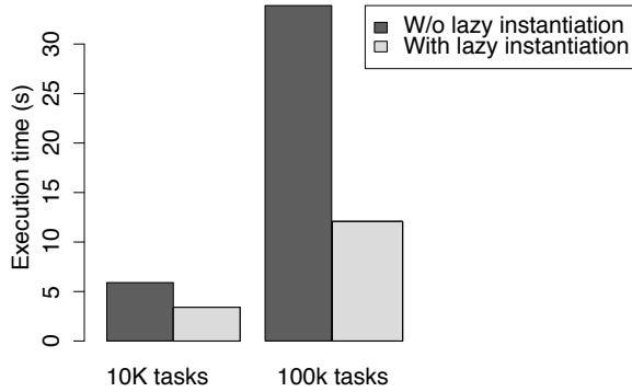
Figure 8: Amount of time spent running a single Spark stage consisting of many tasks without and with lazy instantiation of configuration object.
