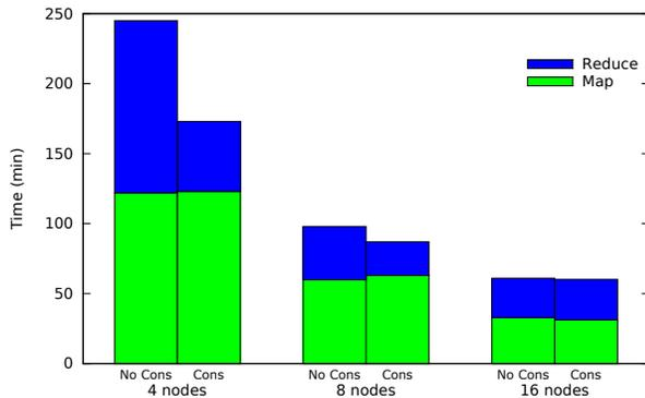
**Figure 5: Spark shuffle file consolidation scaling with Workload 2**
