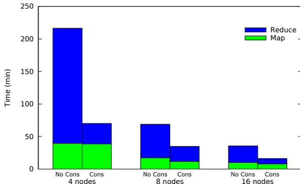
**Figure 4: Spark shuffle file consolidation scaling with Workload 1**
