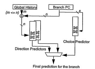
Figure 1: Proposed branch prediction scheme diagram
