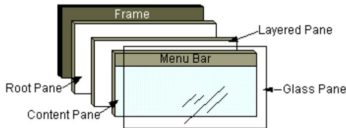
**Figure 5-3: The Structure of a Top-Level Container**
