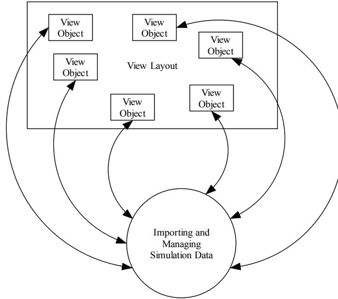
**Figure 2-10: Conceptual Model of View Objects in a View Layout Accessing Simulation Data From the Importing and Managing Simulation Data Component**
