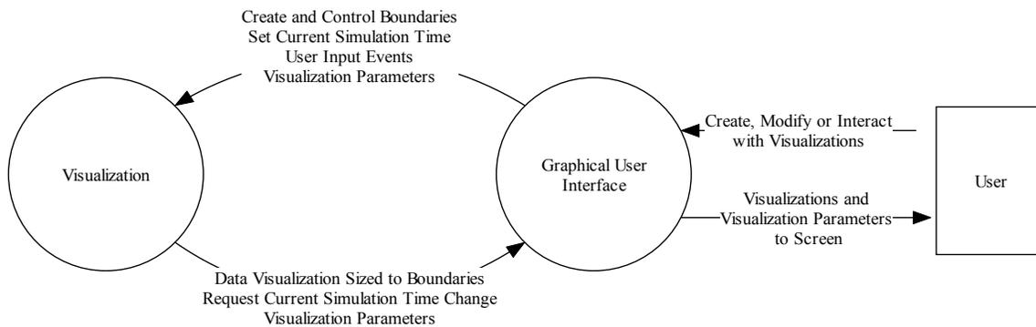
**Figure 2-7: Interface Between the GUI and the Visualization**
