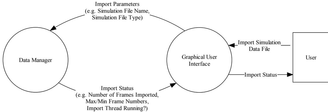
**Figure 2-6: Interface Between GUI and Importing and Managing Simulation Data Components**
