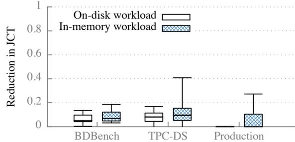
Figure 12: Potential improvement in job completion time as a result of eliminating all stragglers. Results are shown for the on-disk and in-memory versions of each benchmark workload.
