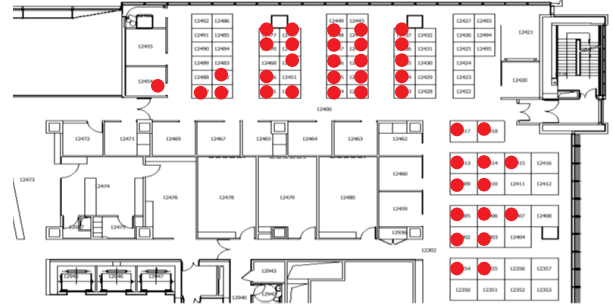
Figure 13. Floor map labeling the deployment location of 41 nodes in the TelosB group.
