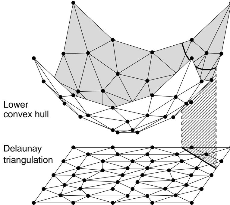
Figure 3: The parabolic lifting map demonstrates that a stabbing line through a Delaunay triangulation is combinatorially related to a two-dimensional cross section of a convex hull.
