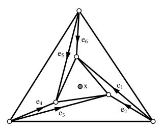
When doing point location on point x in the triangulation above, using the "walking method" as described in Guibas & Stolfi's pseudocode on page 121 of the April 1985 Transactions on Graphics, if we start at edge e1, the algorithm loops forever with the sequence of edges shown. Thus, the algorithm will not always terminate. Note that this is not a Delaunay triangulation.
