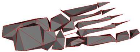
Figure 16: Edge Contractions. 250 face approximation. Bone segments at the ends of the toes have disappeared; the toes appear to be receding back into the foot.
