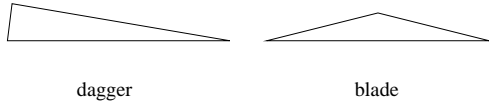
Figure 1: The dagger has one short edge and at least one small angle. The blade has no short edge and therefore one large and two small angles.
