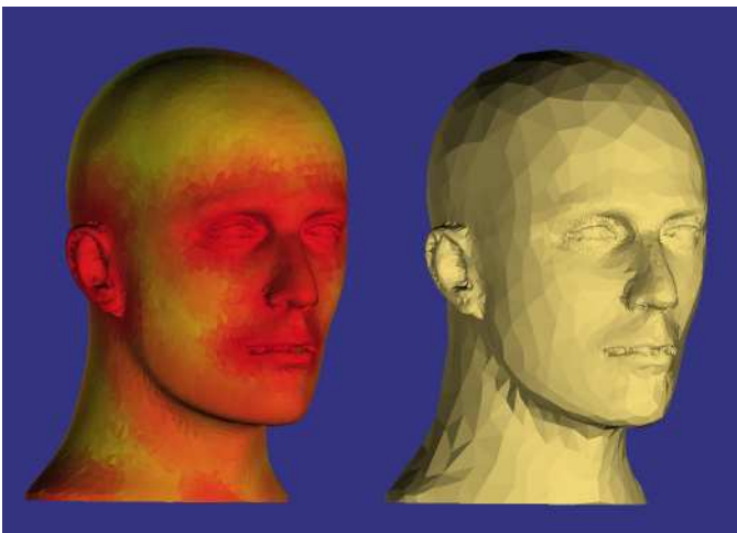
Figure 4. The sampling spacing required to correctly reconstruct a surface is proportional to the distance to the medial axis. On the left is a surface reconstructed from a dense sample. The color represents estimated distance to medial axis—red means close. On the right, we use the estimated distance to thin the data to a .5-sample (meaning that the distance to the nearest sample for any point on the surface is at most half the distance to the medial axis), and then reconstruct. There were about 12K samples on the left and about 3K on the right.
