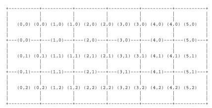
Observe that there is an h-by-(v-1) set of horizontal walls, and an (h-1)-by-v set of vertical walls. In your maze, some of these walls will be present and some will be missing. The walls present are indicated by the arrays hWalls and vWalls, which are an h-by-(v-1) boolean array and an (h-1)-by-v boolean array, respectively. (Exterior walls are numbered according to the same system, but there is no explicit storage for them, because they are presumed to always be present.)
