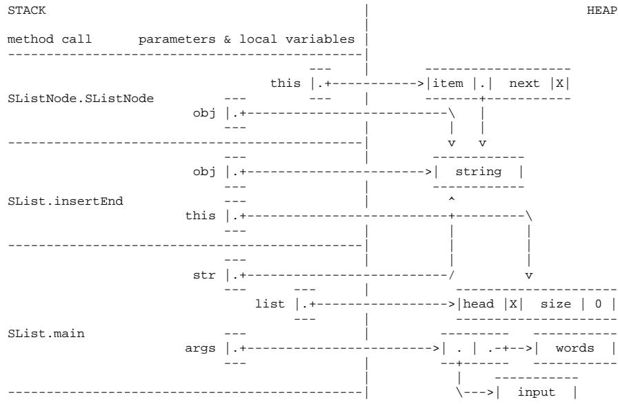
The method that is currently executing (at any point in time) is the one whose stack frame is on top. All the other stack frames represent methods waiting for the methods above them to return before they can continue executing.
