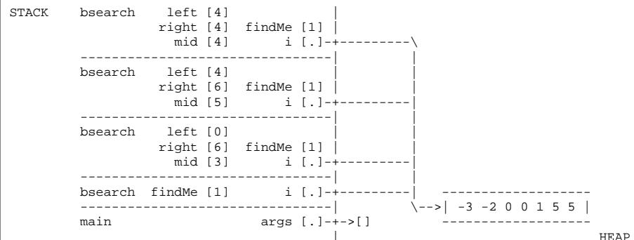
The stack frames appear at right in the figure above. There are three different local variables named "left" on the stack, three named "right", three named "mid", four named "i", and four named "findMe". While the current invocation of bsearch() is executing, only the topmost copy of "left" is in scope, and likewise for "right" and "mid". The other copies are hidden and cannot be accessed or changed until the current invocation of bsearch() terminates.
