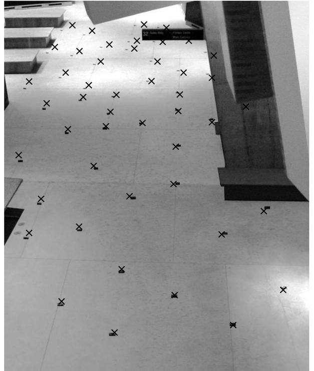
**Figure 2: LaSLAT localization result on a sparser sensor network with 49 nodes in a 10m by 17m environment. Crosses indicate the recovered sensor locations, projected onto the image. The average localization error was 7.5 cm.**
