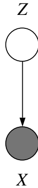
Figure 5.9: A mixture model represented as a graphical model. The latent variable Z is a multinomial node taking on one of K values.
